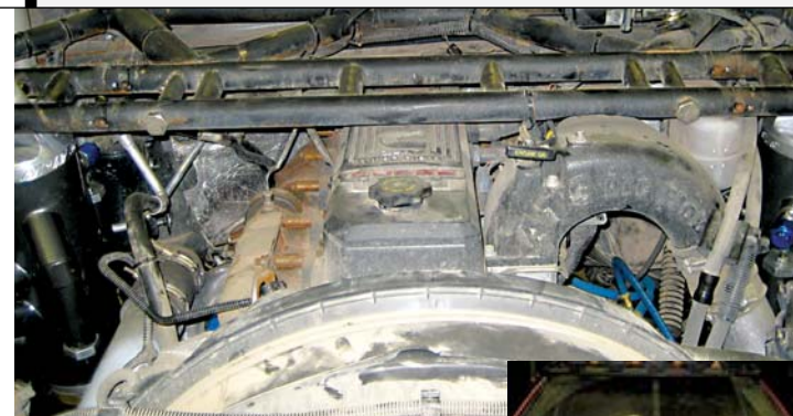
Under that great-looking hood is a powerful Dodge/Cummins turbo diesel engine enhanced with an AEM filter, ATS Diesel manifolds, FASS fuel pump and River City Turbo turbocharger.
